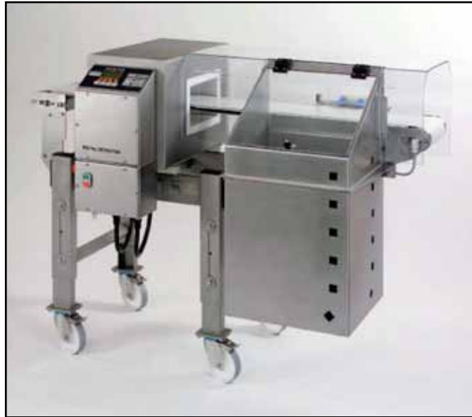
TMDP separation system with conveyor belt, metal detector and reject unit
