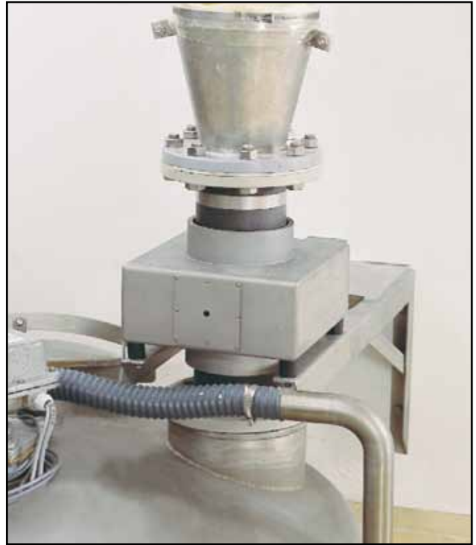
GF tunnel metal detector. Examination of milk powder during bag filling
