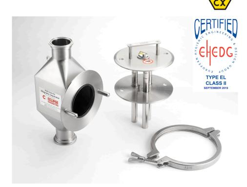
The unit features a double row of magnets on a single assembly high intensity magnetic cartridge. It is secured into its housing by DIN 11853-3 clamps, which ensure even pressure is generated around the O-Ring. The EHEDG Magnetic Separator can be incorporated into lean/dilute phase, conveying lines and gravity pipes in a vertical orientation. A common installation location is at tanker discharge to inspect incoming raw materials.
